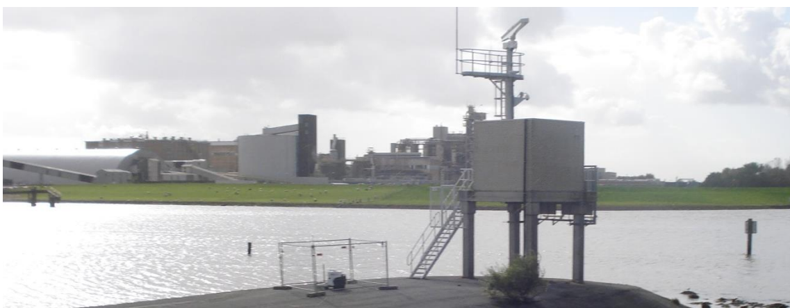
LiDAR deployed to complement met mast 4 km away [Project Reference: Delfzijl Noord]
